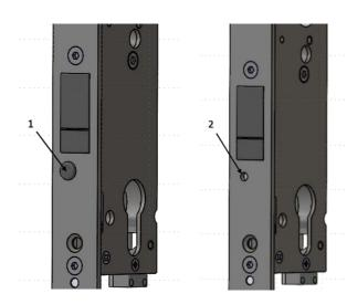
Before programming and deleting transmitters, the cover (1) underneath the receiver unit must be removed.
